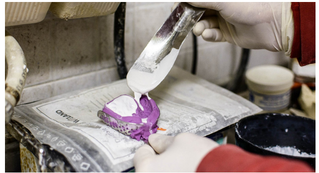
After receiving a dental impression from a dentist, OpLab used to create a plaster cast.
