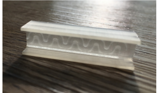
The fluidic channel is visible inside the device – a straight channel down the side and a snaking path through the middle.
