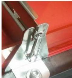
7. Red Slide Plate sticking (located underneath the Vat) – [Clean inside rails with Isopropyl alcohol](#).
