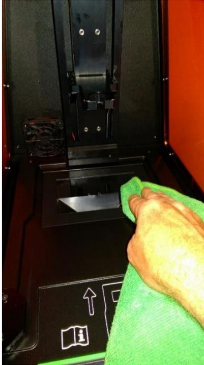
Large spills and resin drips can be cleaned using Isopropyl Alcohol (85% min), but the final cleaning of the glass optics must be done with a clean, dry microfiber cloth. Do not use paper towels.
