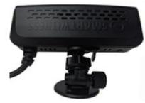
IMPORTANT: Make sure the glass is clean and dry before attaching to the windshield, holding the camera in position for 30 sec. with firm pressure. The glass temperature should not be too cold or hot. Please install the camera in moderate temperature (between 50°F ~ 80°). The distance angle from the driver's face should not exceed 20°
