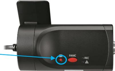
There will be a beep and LED light blink to indicate the G-Sensor calibration has registered.
