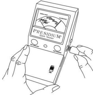
1. Insert the probe pen into the socket at the side of the tester before turning on the unit.
