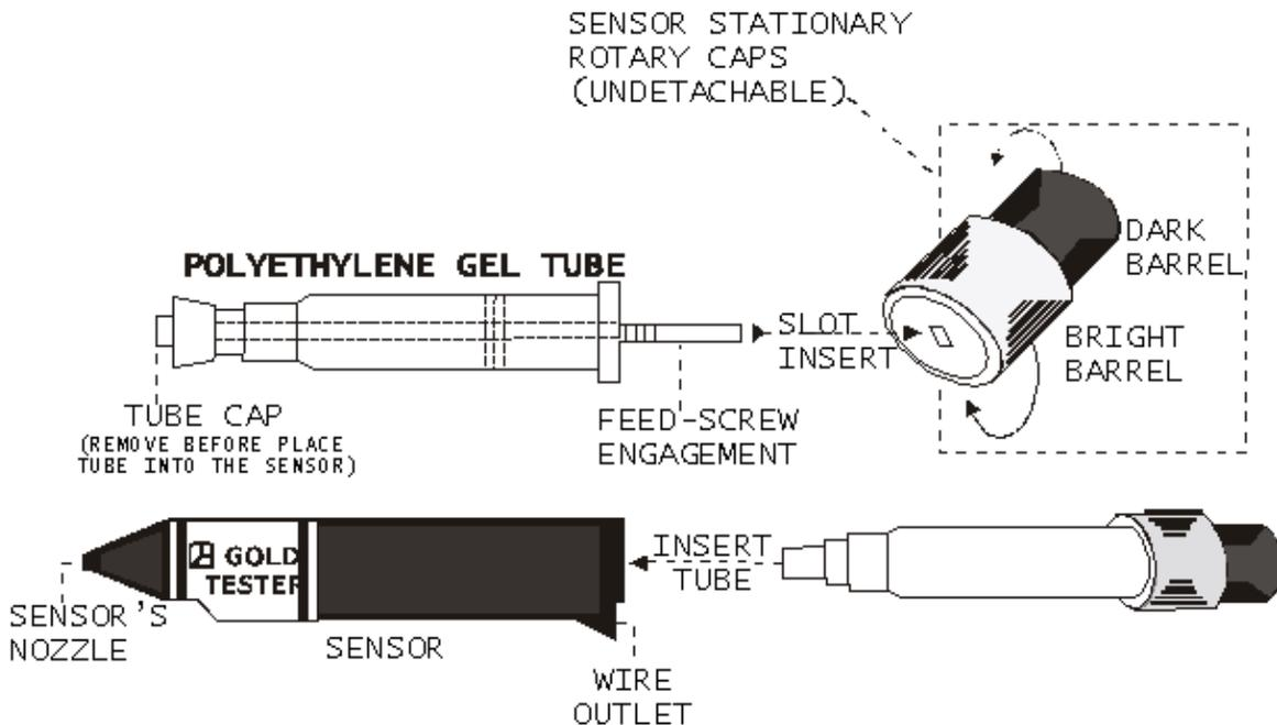
*Sensor and Polyethylene Gel tube*
