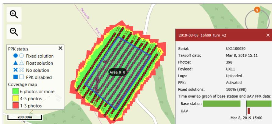
Figure 1: Improved flight information window. In this example, two RINEX files were declared in the PPK base station window, but they happen not to overlap. Hopefully, the second one starts slightly before our flight, which is thus fully covered.
