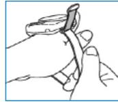
Attach PULSOX 300i to the arm by inserting your hand through the Wrist Band
