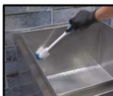
Immerse a clean brush in sanitizing solution and clean the entire ice chute. Allow to air dry
