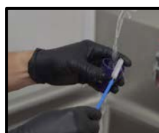
Brush the nozzle with a dedicated soft bristle flexible brush using warm water
