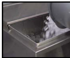
Fill the ice bin with clean ice. Note: The Ice Bin must be a minimum of 50% full for 20 minutes for proper dispensing temperature
