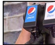
Remove all nozzles and diffusers, separate if necessary
