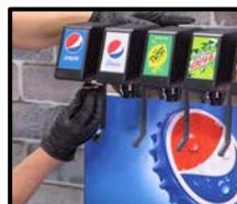
Replace the nozzles and diffusers back into the bottom of the valves
