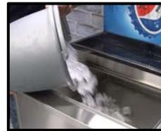
Fill the ice bin with clean ice. Note: The Fountain Ice Bin must be a minimum of 50% full for 20 minutes for proper dispensing temperature
