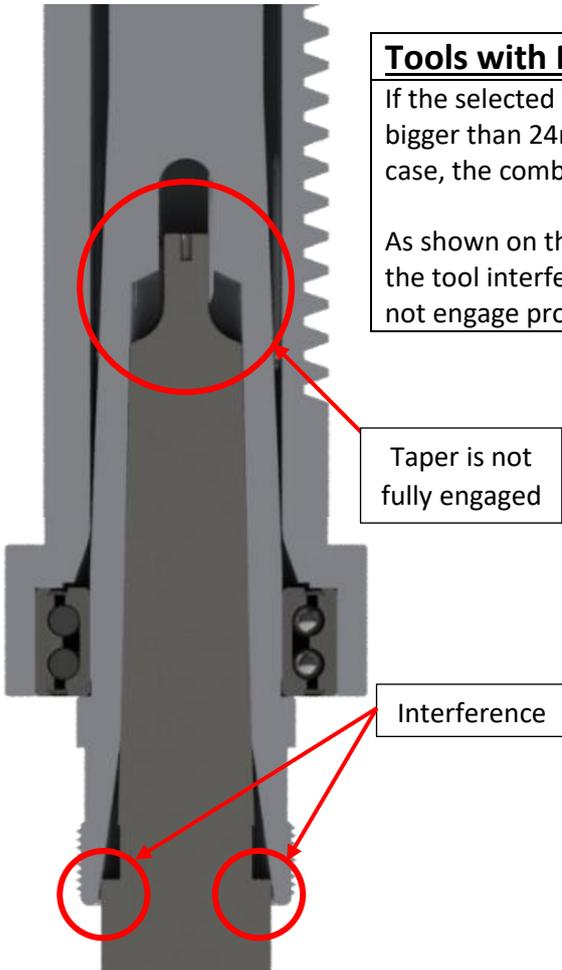
If taper tool is not compatible with the spindle
