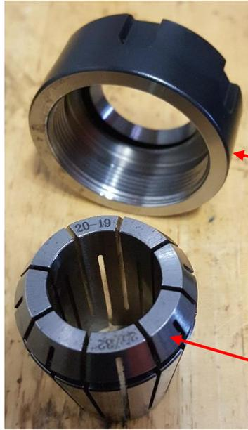
ER32 collet hold the cutting tool by using 2 main parts; collet and collet ring. The collet ring squeezes the collet ring which then squeezes the cutting tool therefore holding the tool in place.
