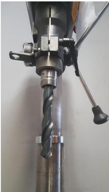
*1inch drill bit with MT3 mounted directly into the spindle*
