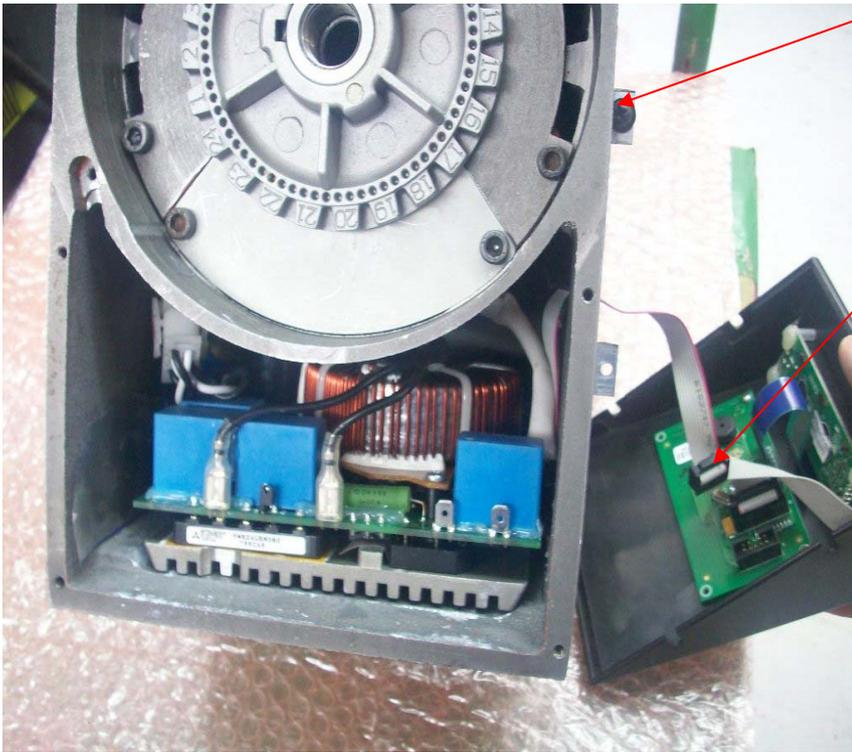
Unfasten these a few turns to release the control cover. The ribbon will be connected and will have a blob of glue bonding the plug and receptacle together. The glue can be pulled off and the ribbon plug removed. Feed the ribbon plug back through the hole on the side avoiding any scraping on the ribbon.
