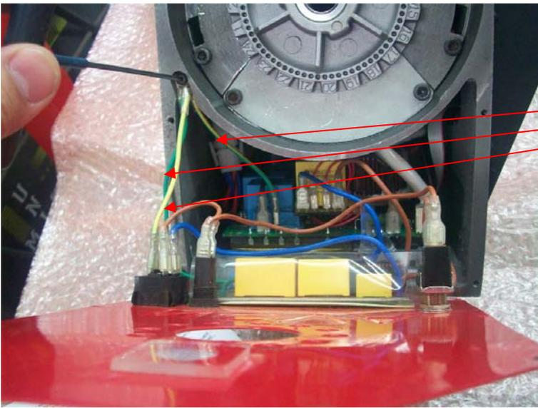
The three earth wires must be connected together and be fastened into the inside of the headstock casting.
