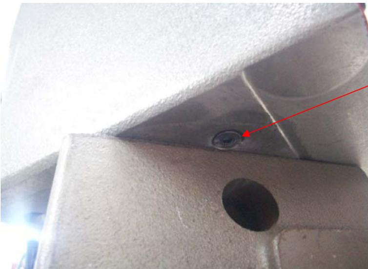
The front screws may be difficult to reach. To help the heat sink has been chamfered to help locate the screw into the thread.
