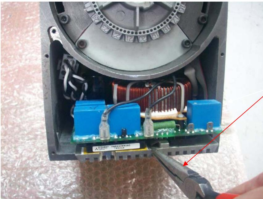
Pliers to hold onto the heat sink. Be careful not to touch any components and clamp only onto the aluminum heat sink.
