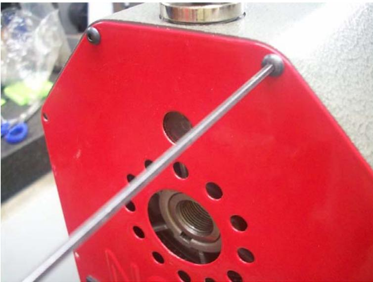
9. Position the control board panel on its bracket and fasten the 4 screws on the sides.
