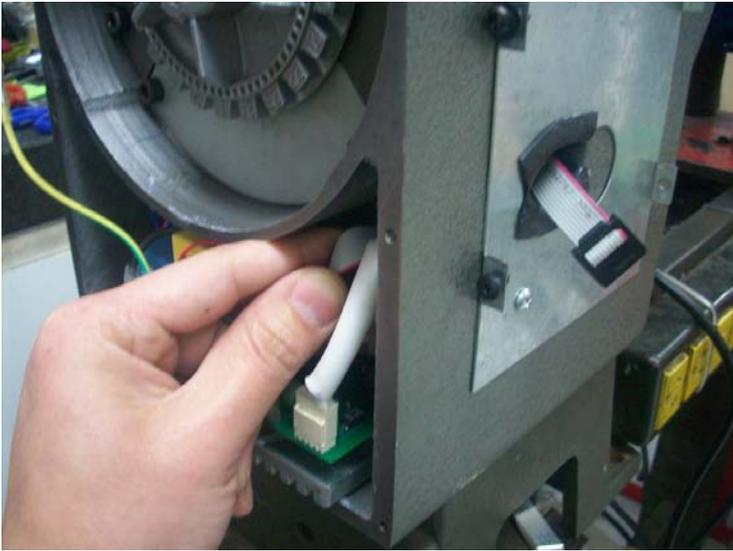
Feed the 10 pins ribbon from the new control panel through the hole on the side of the headstock and feed the control board all the way in and then push the 6 stator wires back in place.
