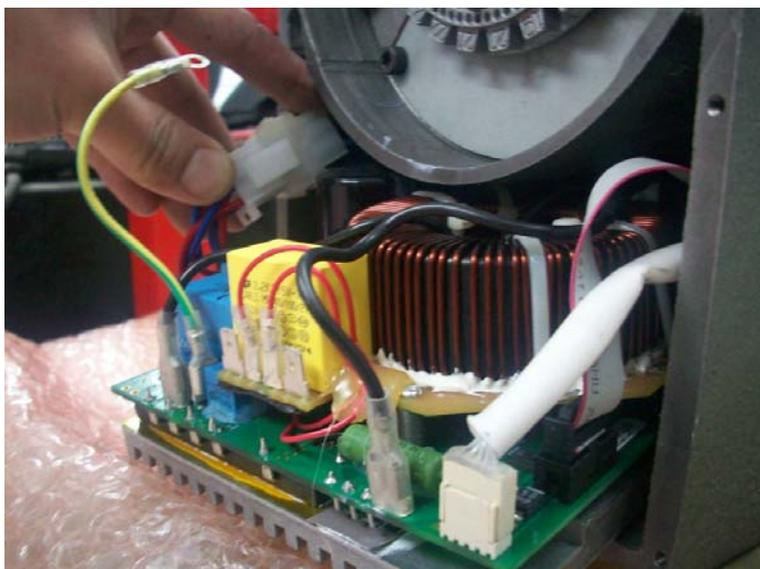
Feed the control board  $\frac{3}{4}$  of the way in and plug the 6 pin stator wiring plug into the corresponding plug on the control board. Attach the sensor cable and the ribbon cable into their corresponding sockets on the control board.
