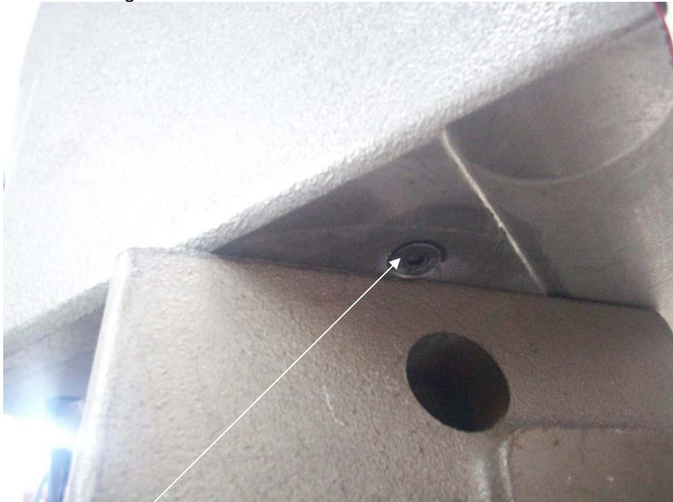
Screw exposed by swivelling head stock around
