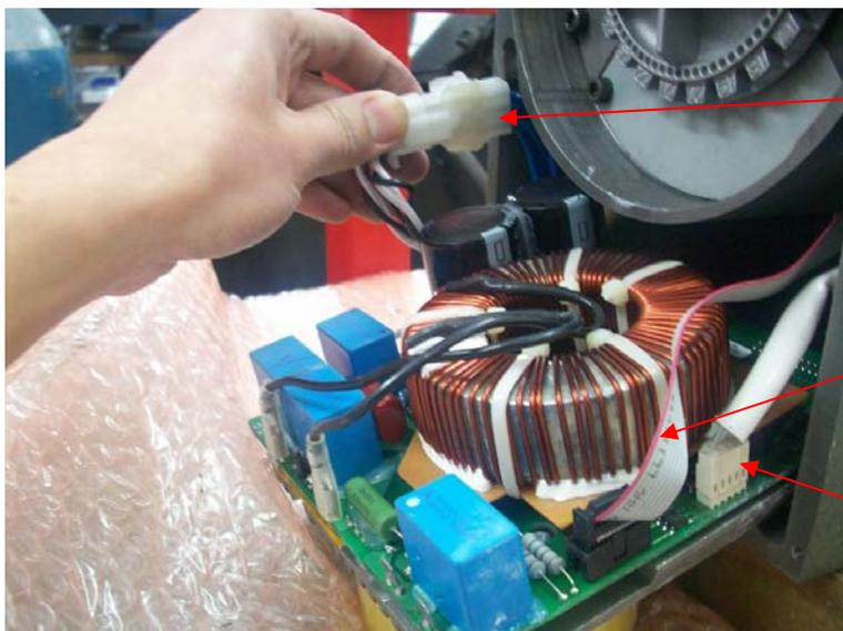
Disconnect the 6 pin white plugs thus separating the stator wiring from the control board.
