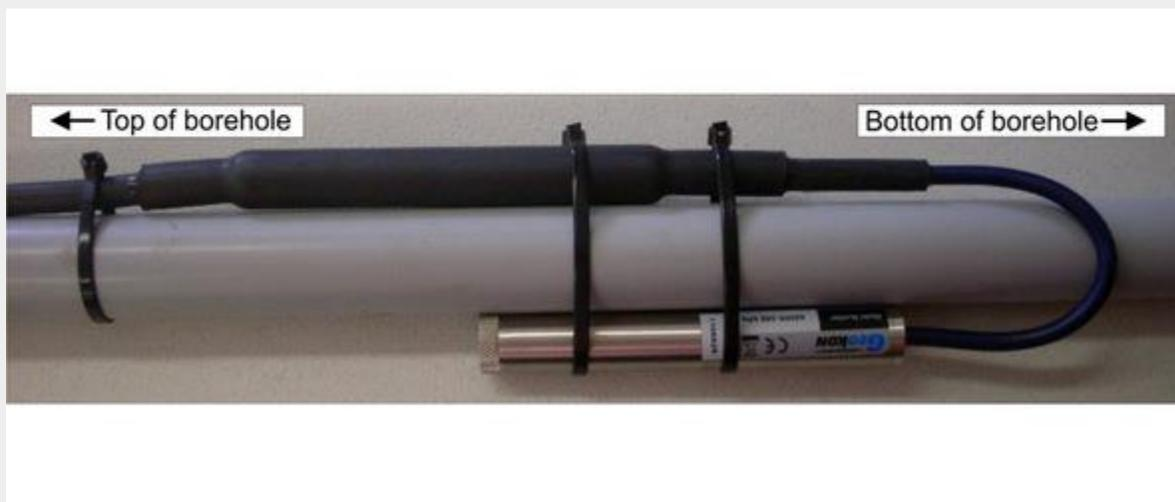
Figure 4.1: SAAPZ mounted to PVC conduit
