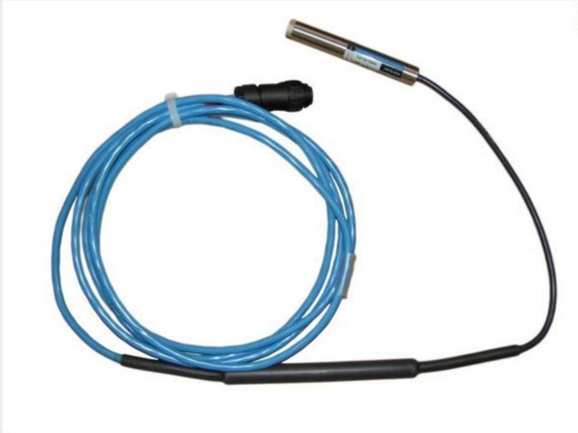
Figure 2.1: SAAPZ Unit containing the SAAPZ processor and digital temperature sensor. (A) Vibrating wire piezometer element, (B) Processor pod
