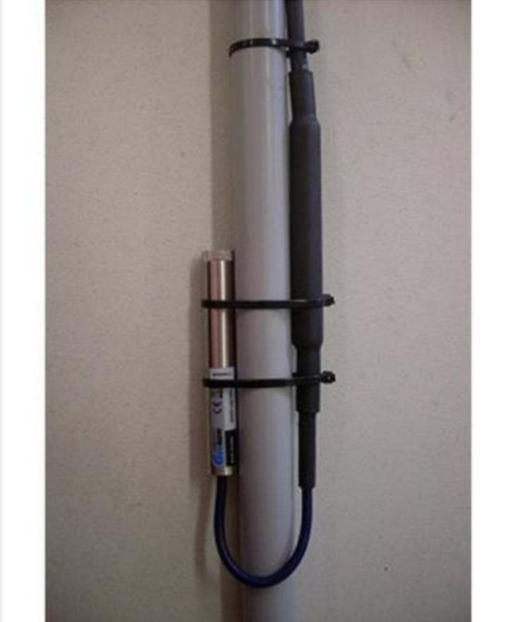
Figure 1.1: PZ1\_vw sensor mounted to 27 mm ID PVC conduit (SAA inside). The VW piezometer (made by Geokon) is on the left and the Measurand microprocessor-based interface is on the right
