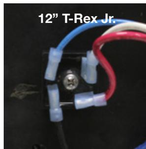
5. Reattach all four wires to the posts of the rectifier in the positions shown. **NOTE:** Position of the red and blue wires is dependent on the T-Rex model you own, depicted above.
