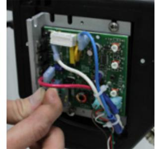
1. Remove black rear panel cover with 1/8" Allen wrench. Using a Philips screwdriver, loosen screws pictured above to remove blue front panel.
