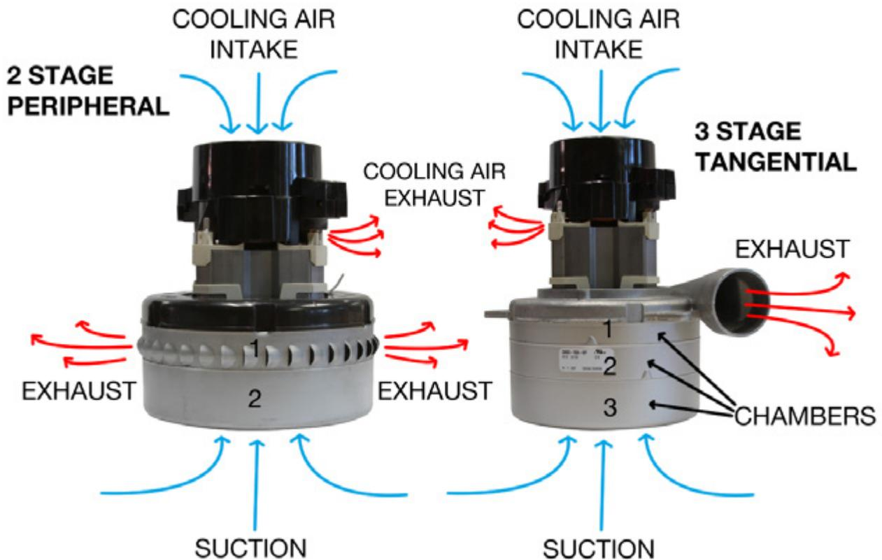
A vacuum motor has vacuum **chambers** (or stages). Each stage is a fan in a sealed compartment. You can usually tell how many stages a vacuum has by counting the number of chambers. Chambers make up the bottom portion of the vacuum motor and resemble layers of a cake. The more stages a vacuum has, the more powerful the suction.
