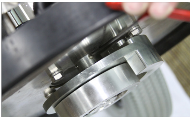
2. Loosen the four set screws holding the flywheel onto the shaft using a 1/8" Allen wrench and slide the flywheel assembly off the shaft.
