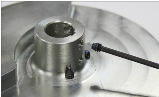
4. Apply blue threadlocker to the two small set screws (3) and thread them into the holes where the key slot is. They do not need to be threaded in very far. Make sure they don't stick out into the key slot.
