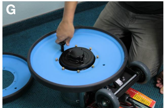
**Step 4:** Slide the bolts and washers into place and hand-tighten. Follow up with your 7/16" socket or wrench, tightening in a star pattern (**Figure G**).
