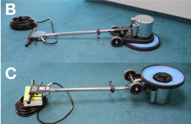
**Step 1:** Lower the handle all the way to the floor (**Figure B**). Flip the machine over and prop up the handle (**Figure C**).
