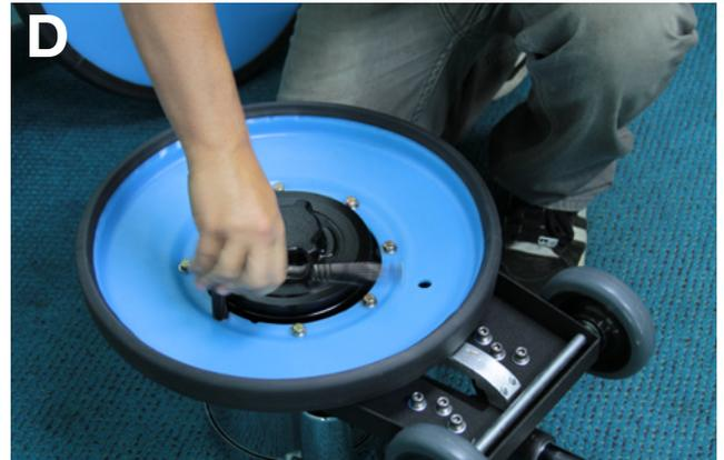
**Step 2:** With a 7/16" socket or wrench, remove the 8 bolts holding the shroud in place. Remove the shroud (**Figure D**).
