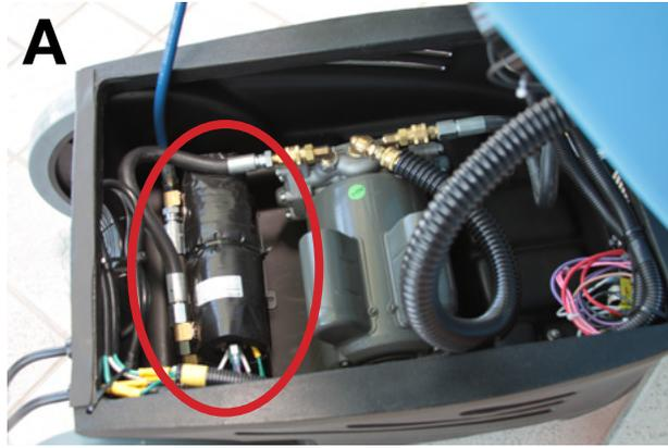
**Step 2:** Press the small white and yellow button on the heater. This will reset the heater. If the unit has more than one heater, make sure to reset both heaters (Figure B).
