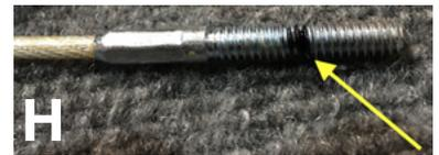
**Step 12:** Screw in this cable end to the locking piston, up to the mark on the threads previously made with the Sharpie. (Figure J)
