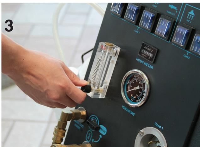
**Step 3:** Set meter to desired ratio. Meter is measured in GPH (Gallons Per Hour), which indicates how many gallons per hour of concentrated chemical will be metered.
