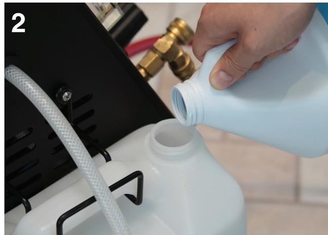
**Step 2:** The chemical bottle hangs on a holder on the side of the machine. Fill it with the desired chemical concentrate you wish to mix into the clean water tank.
