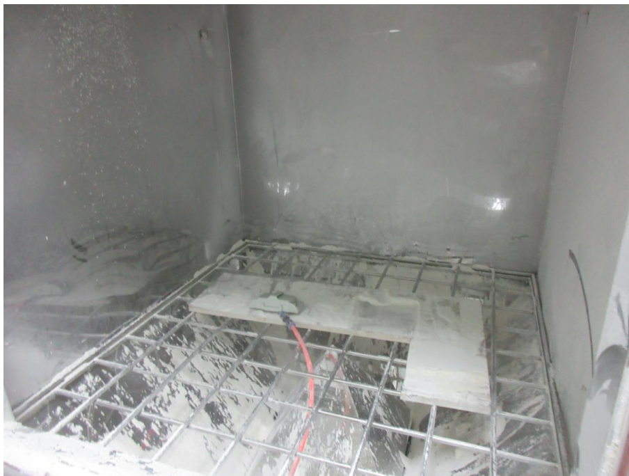
Photo 2: IP6X test of Reindeer
