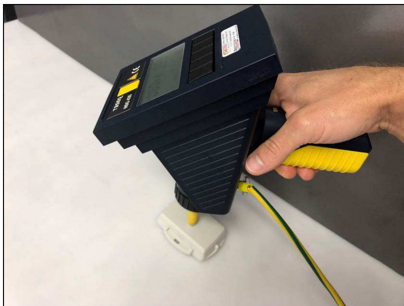
EN / IEC 61000-4-2: ESD immunity test set-up
