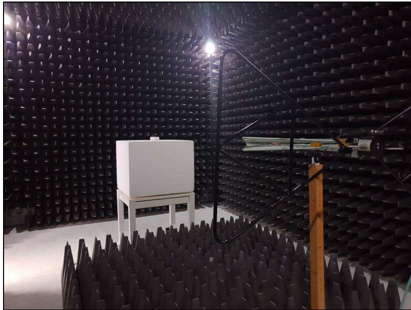
EN 55032 / CISPR 32: Radiated emissions test set-up
