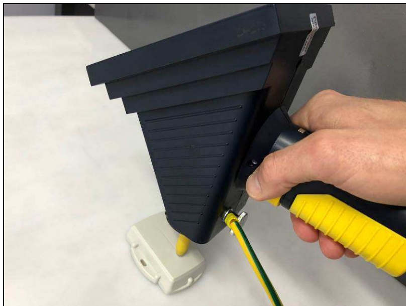
EN / IEC 61000-4-2: ESD immunity test set-up
