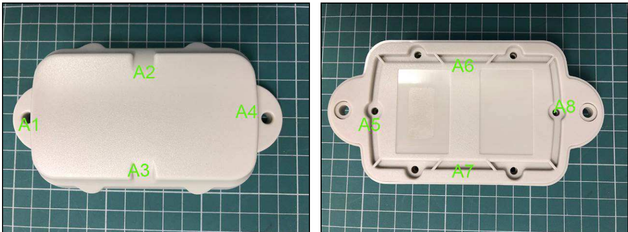
Figures 4 & 5: ESD discharge application points
