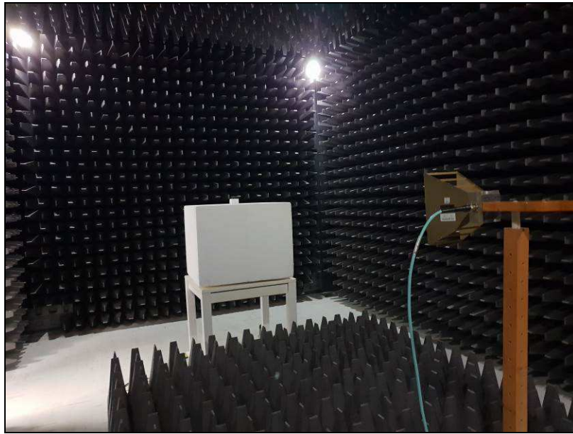
EN 55032 / CISPR 32: Radiated emissions test set-up
