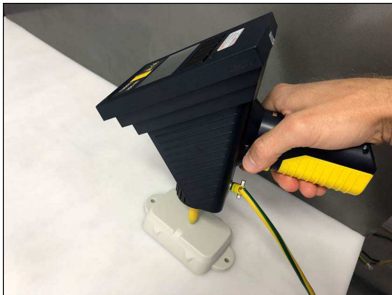
EN / IEC 61000-4-2: ESD immunity test set-up
