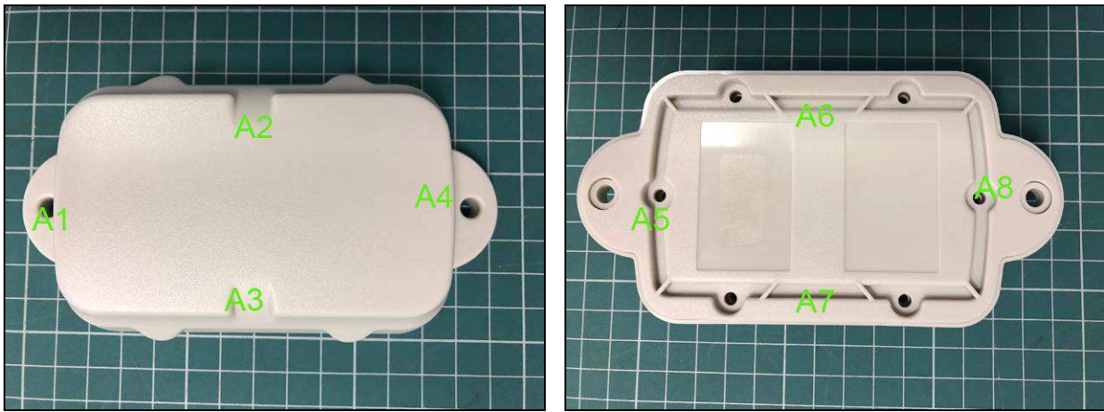
Figures 4 & 5: ESD discharge application points
