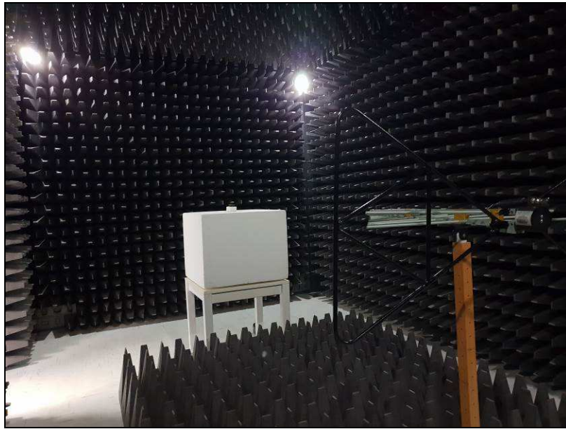
EN 55032 / CISPR 32: Radiated emissions test set-up
