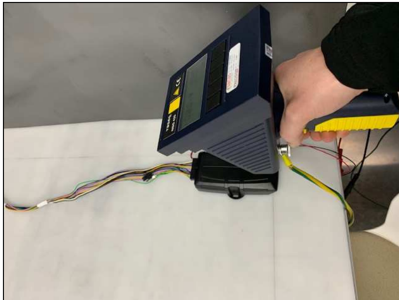
EN / IEC 61000-4-2: ESD immunity test set-up
