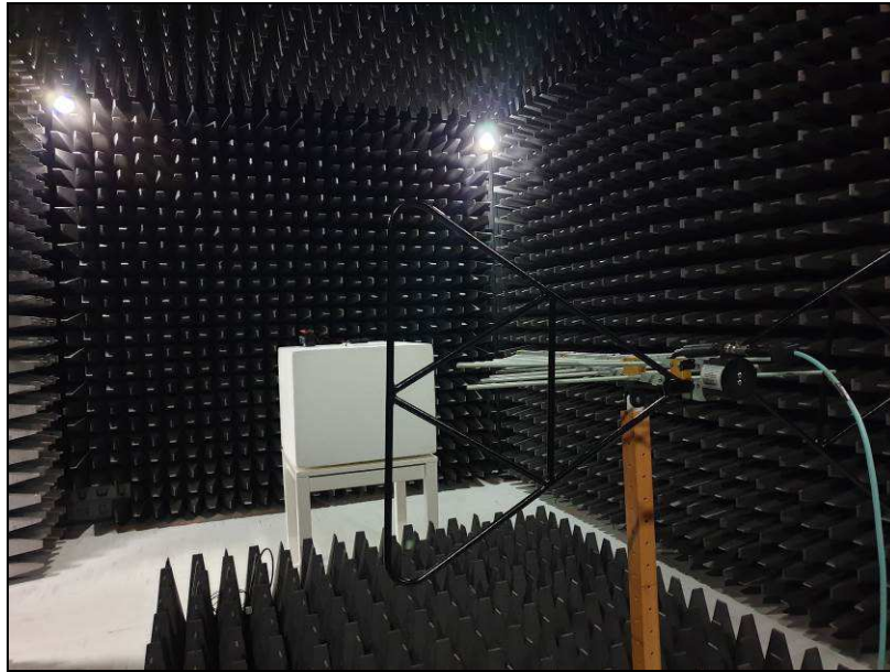
EN 55032 / CISPR 32: Radiated emissions test set-up
