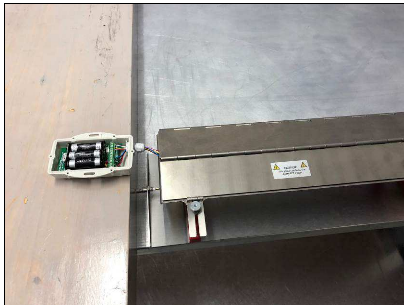
EN / IEC 61000-4-4: Fast transient / burst immunity test set-up
