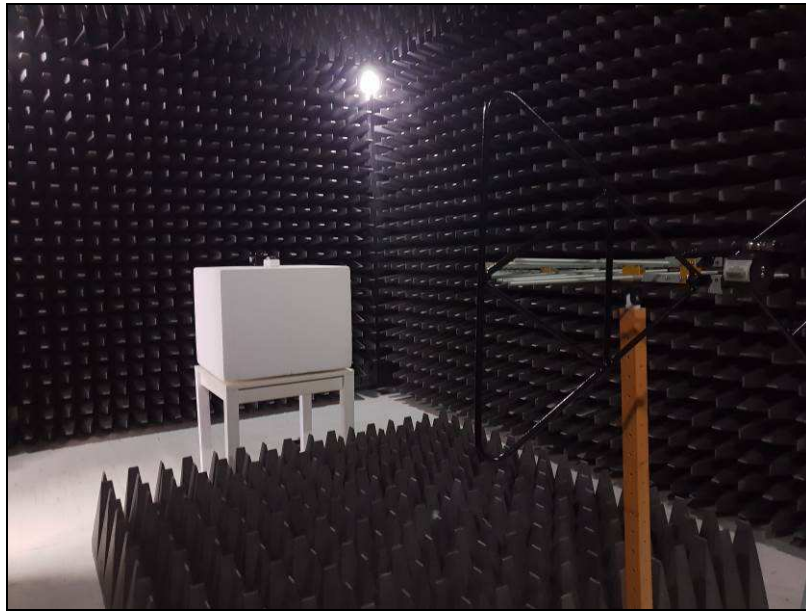
EN 55032 / CISPR 32: Radiated emissions test set-up
