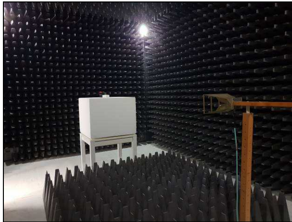
EN 55032 / CISPR 32: Radiated emissions test set-up
