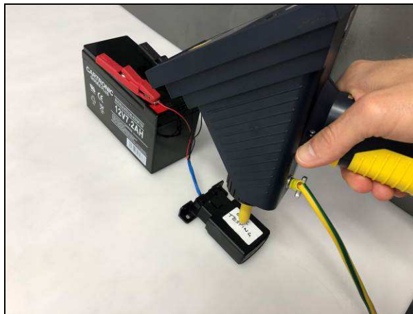
EN / IEC 61000-4-2: ESD immunity test set-up
