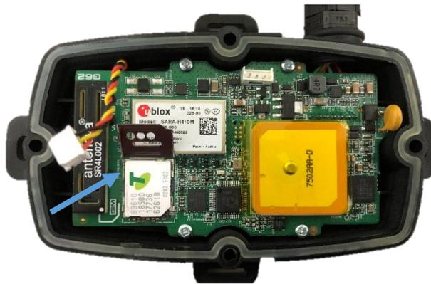
1. The SIM holder is located on the top side of the main PCB.
