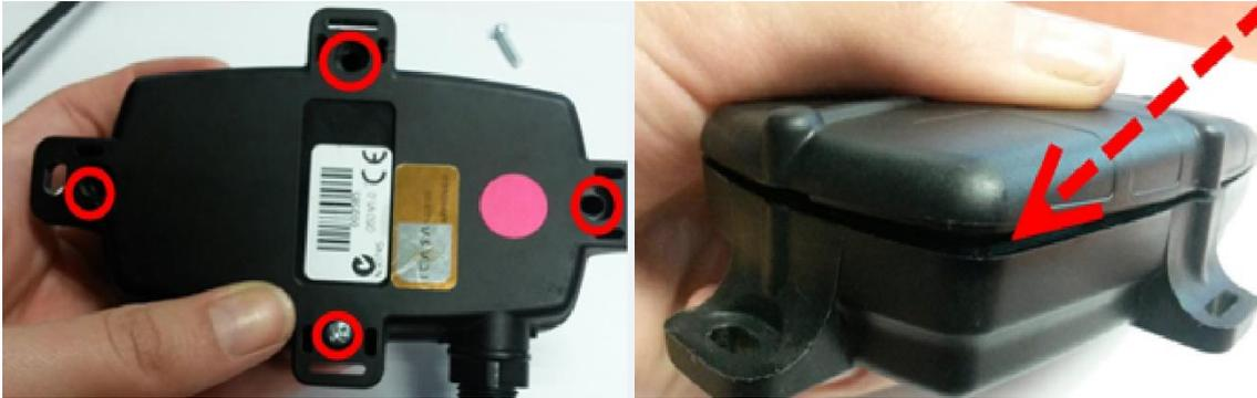
Ensure that the main PCB is secured to the housing with the 4 small PCB screws and that the SIM is inserted as above. Ensure that the device is online before sealing it.
