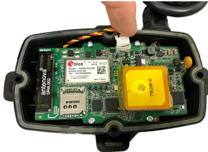
The battery should be provided disconnected inside the housing. The battery plug is a three-way connector on the top side of the PCB.
