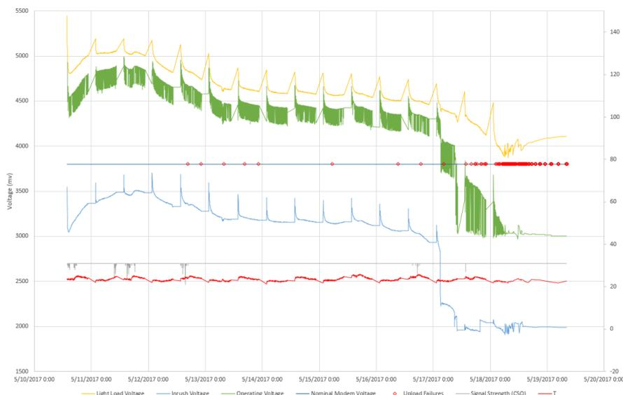
At room temperature, the open circuit battery voltages (sampled after the 3 hour sleep) produce graphs similar to:
