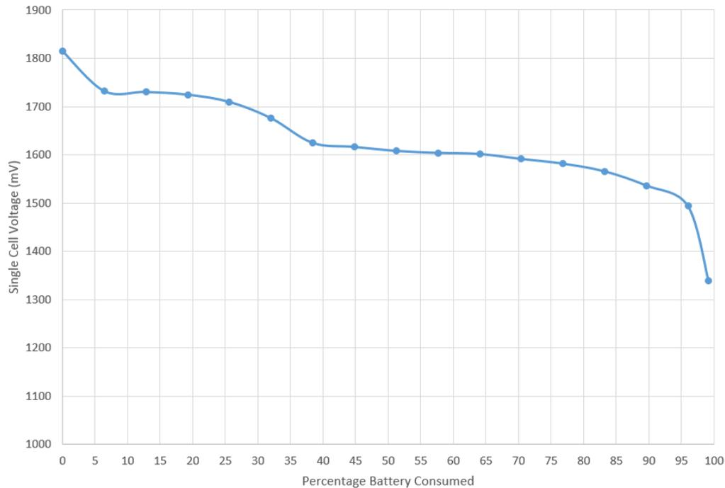
At lower temperatures (< 10), the voltage is not able to recover, and the graph becomes temperature and duty-cycle dependent. This graph was captured at roughly 5° C:
