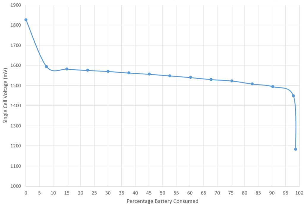
In the field, the Oyster Cellular reports the maximum voltage sampled in the last 36 hours. If temperatures are moderate or hot, and the Oyster is not in continuous operation, the state of charge can be estimated from the room temperature graph.
