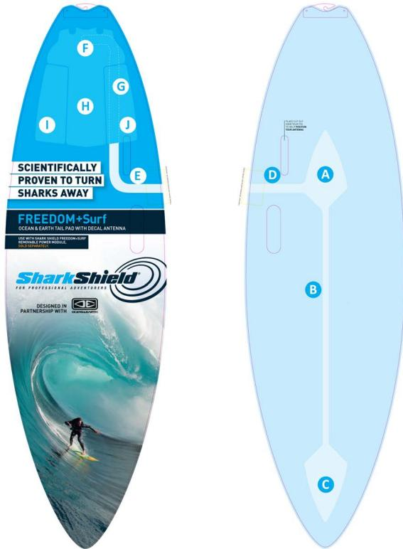
**Step 3.** Slide the antenna down the board and ensure the part of the ribbon cable that wraps around the board rail to the tail pad is no more than 25mm (1") in front of the most forward left fin. Now peel off the backing of the tape that has an **A** on it for the bottom electrode. Apply.
