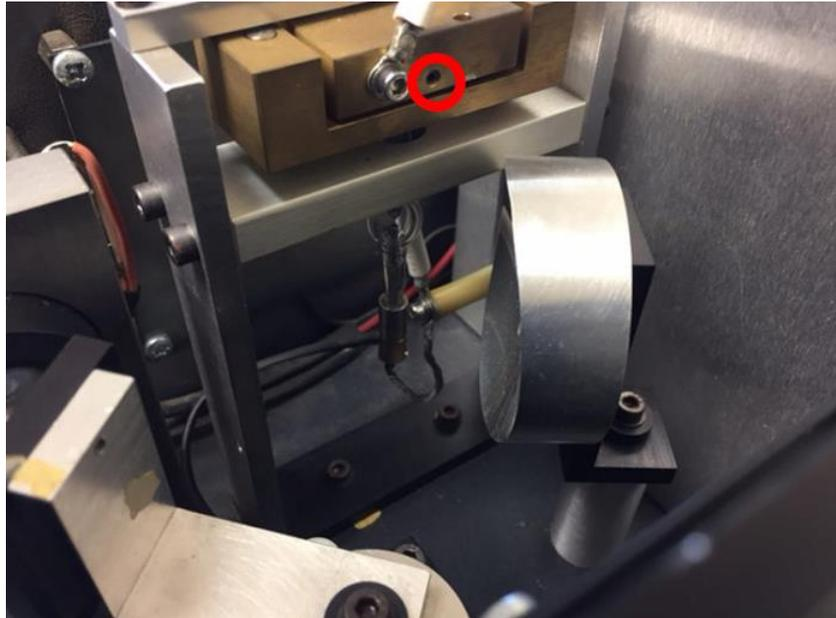
*Figure 6: Grub screw that releases the top of the xenon lamp*
