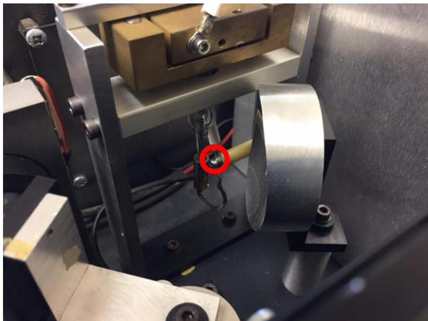
*Figure 7: Remove this screw to remove the cable connecting the xenon lamp*
