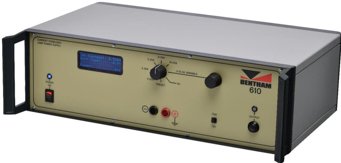
The Bentham 610 is a constant current power supply designed for use with stabilised light sources and calibration standard sources. The unit is capable of sourcing 10.4 A DC current at a voltage of up to 26 V.
