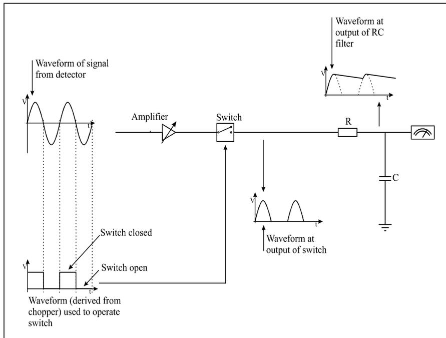
Figure 8: Synchronous Filter
