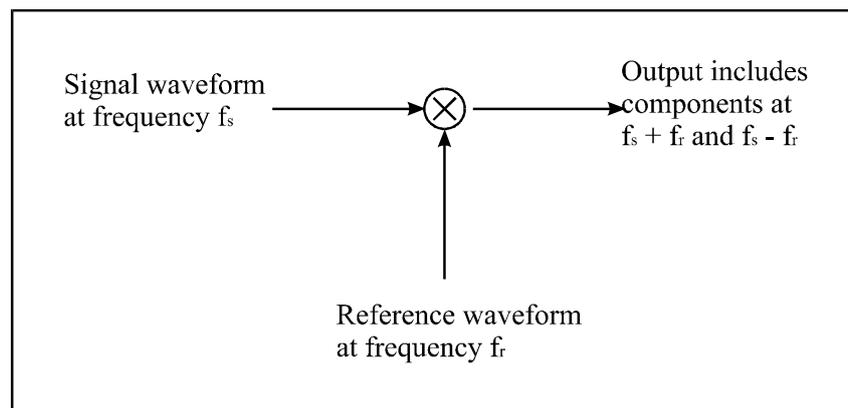
Figure 9: Alternative visualisation of phase detector
