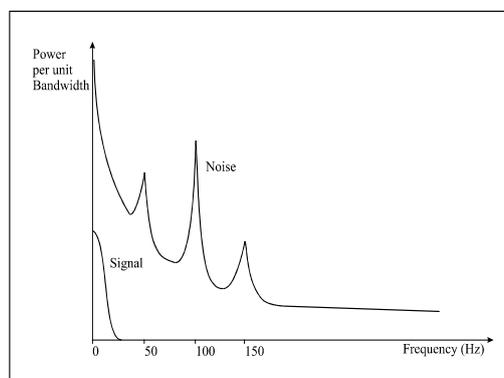
Figure 4: distribution of noise and signal power from the optical detector in terms of power per unit bandwidth as a function of frequency
