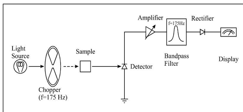
Figure 7: A standard measurement system using lock-in amplifier
