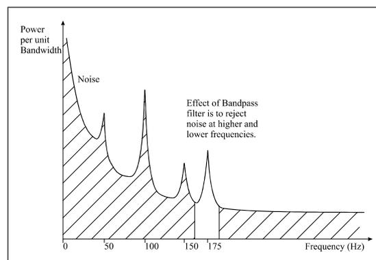
We can do this by placing an optical chopper, which will periodically interrupt the light between the light source and the detector. The diagram below shows the detector output spectrum in this new situation with the chopper running at 175Hz.
