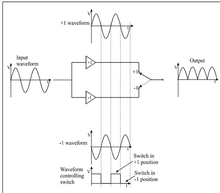
Figure 10: Rectifier operation
