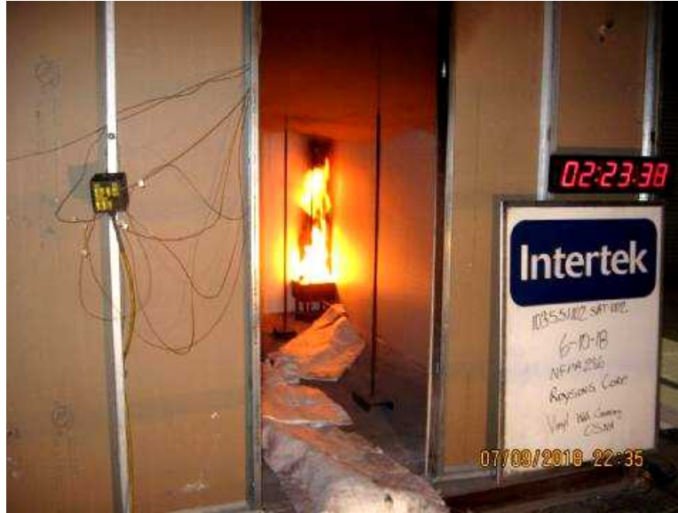
Photo No. 3 Flame spread/smoke density at 40kW
