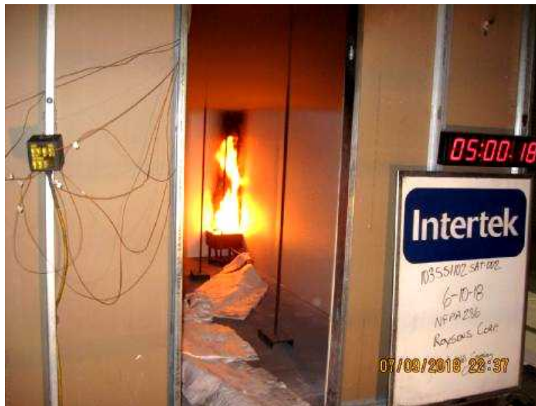
Photo No. 4 End of 40kW exposure
