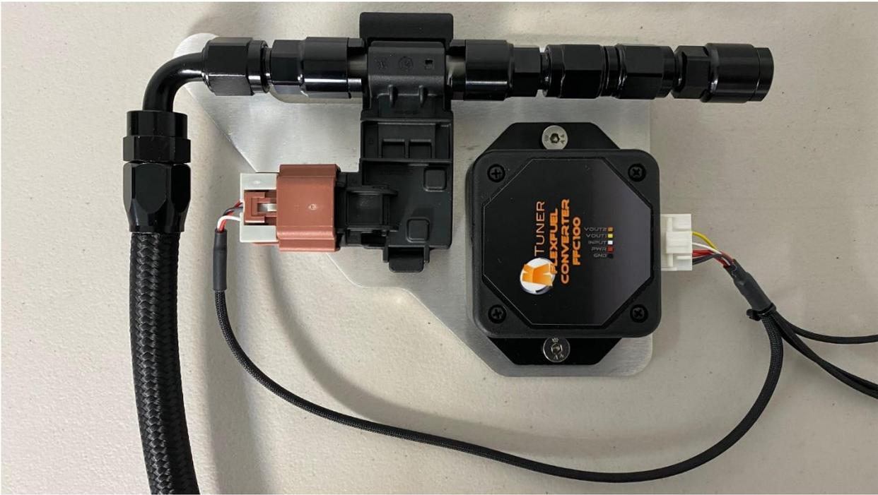
**\*\*\* IMPORTANT \*\*\*** Next take the 5/16 SAE quick disconnect (with plastic) and install that into the 45 degree hose end and tighten. It will be difficult to tighten later if you do not do it before connecting it to the HPFP (high pressure fuel pump)
