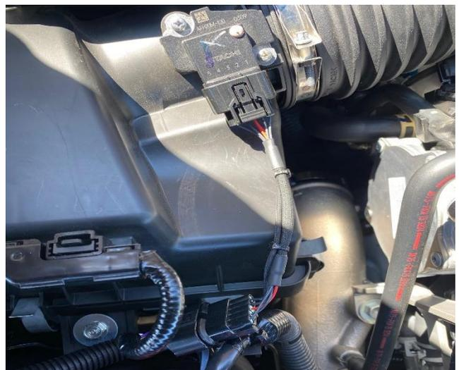
The longest branch is to be routed down to the ECT2 sensor which is on the bottom of the radiator on the drivers side. You will most likely need to remove the flexible intake to gain access to that area. Disconnect the factory ECT2 connector and plug that into the male connector on the harness. Again, route and secure the wire in an appropriate fashion.
