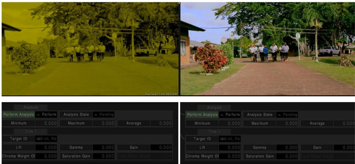
When it finishes the **Analysis** parameter will automatically change to **“Completed”** state and the image output sent to the target display will be already calibrated. The above picture shows a Before (Analysis pending) / After analysis example.
