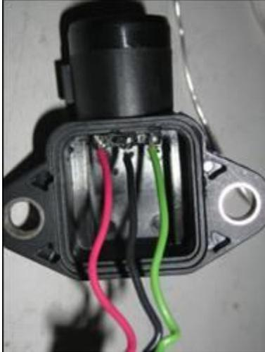
Next solder the 3 wires to the map sensor board. On the back of the board, you should see the number “340166” and if you have the board facing you so that number reads correctly, the wire color order to solder to the board from left to right should be Red (5v), Black (ground) and Green (signal). It should look like the following picture:
