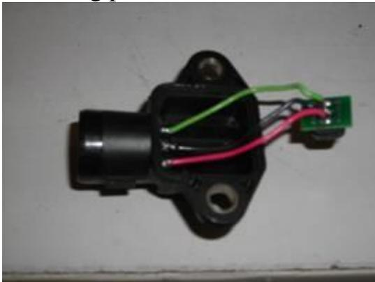
Next take a 3/32” Drill bit and slightly enlarge the hole for the sensor in the bottom case piece. This will allow the sensor nipple to snugly fit in the bottom case piece. Do not drill to big...just enough for the sensor to fit in the hole securely. Fit the sensor in the bottom piece, it should look like this:
