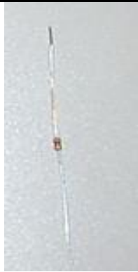
10K resistor (Brown-Black-Orange-Gold) are the stripes on this
