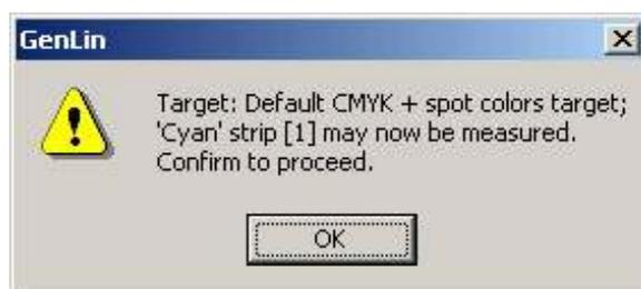
Arrange the target in the direction of the arrow with the first (Cyan) strip under the measuring head and slide the target under the head until it stops. Click OK and feed the target gently through the reader.
