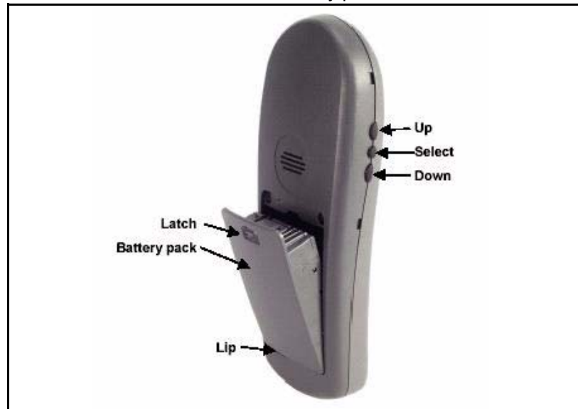
Figure 5 WLAN Handset 2210 and 2212 battery pack location
