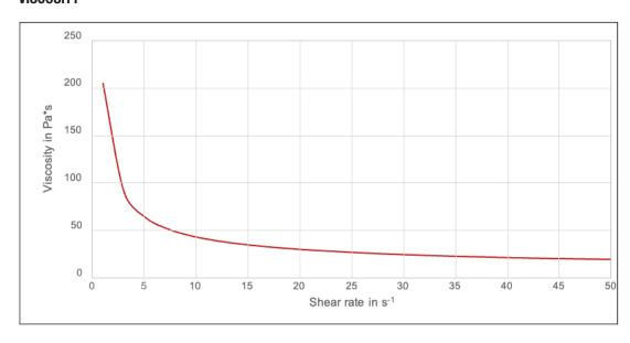
Measuring conditions: Rotational viscometer, 25mm plate, gap 0.5mm
