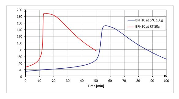
**Measuring conditions:** 100g mixture conditioned at 5°C and measured in climate chamber at 5°C 50g mixture conditioned at RT and measured in fume hood at RT
