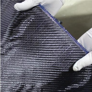
50" Wide. Our most popular carbon in prepreg form. Identical to part# 1069, this prepreg offers the advantages of pre-impregnation of an epoxy resin system. The material can be stored, shipped and handled at room temperatures and is cured using ramp up schedule requiring at most 310°F. Resin content 37.00% +/- 3%.
