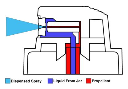
When the button is pressed, propellant and liquid are mixed and dispensed as a spray at the nozzle by action of the venturi effect. Liquid from the jar is pulled up the tube as propellant travels across the holes in the red insert (inside the button). The propellant and liquid do not mix prior to being dispensed out of the nozzle.
