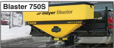
When you need to control the flow of any material, the Meyer Blaster is the tailgate spreader for you. Compatible with ½-ton and larger pickup trucks with a two-inch receiver or tractors with a three-point hitch, the Meyer Blaster comes in two sizes: The Blaster-350 is available in a 6.5-cubic-foot capacity and the Blaster-750 features a 12.8-cubic-foot capacity.
