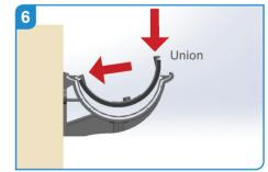
Ensure that all fixing surfaces are clean and dry. Placing the union into the groove in the rear face of the gutter and clip down into place on the front edge.
