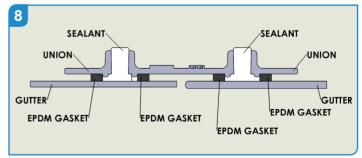
Ensure you apply the sealant gently to ensure the void is fully filled.
