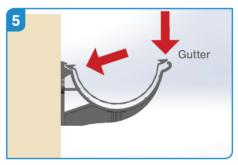
When fitting outlets and angles tuck the rear face of the gutter underneath the roof finish. Locate the gutter into the fascia bracket and then clip the front edge down into position.
