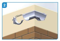
Image 2 shows the bracket positioning for the angle and bracket to take the gutter length.
